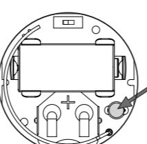
The LEDs of the new wireless input module flash green once first, then light up yellow for one second and then flash red four times. As soon as the LED goes out after that, the connection can be set up.
