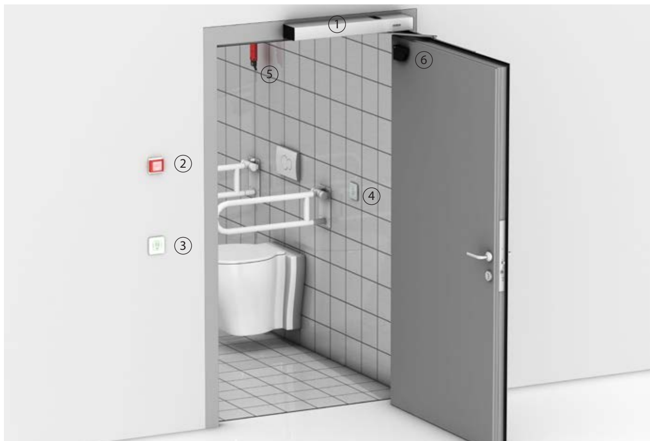
1 = Swing door drive | 2 = Emergency shut-off switch (recommended installation height: 1600 mm) | 3 = Non-contact proximity switch (flush-mounted) | 4 = Non-contact proximity switch (surface-mounted) | 5 = Pull switch emergency call | 6 = Laser scanner
