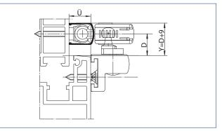
D = Distance from outer edge of leaf to centre of link arm I Y = Upper clearance I  $\ddot{U}$  = Overlap height Diagrams illustrate the area of application of the leaf bracket variants
