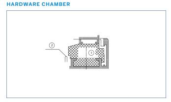
1 = Space requirement for F 1200 components I 2 = Seal end face
