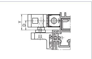
D = Distance from outer edge of leaf to centre of link arm | D\* = Distance from outer edge of leaf to centre of link arm (preferably 17 mm) | Y = Upper clearance
