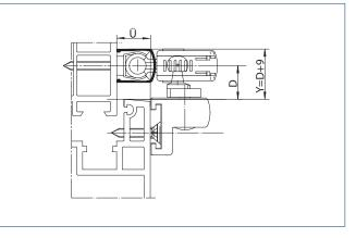
D = Distance from outer edge of leaf to centre of link arm I Y = Upper clearance I  $\ddot{U}$  = Overlap height Diagrams illustrate the area of application of the leaf bracket variants
