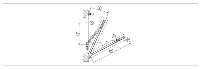
1 = Safety opening width | 2 = Length when closed | 3 = Safety position | 4 = Cleaning positioning | 5 = Leaf height
